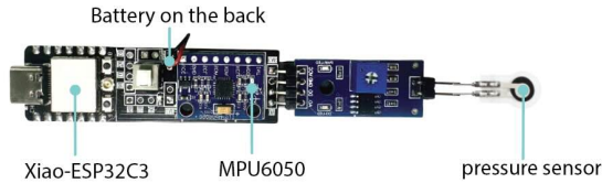
Figure 2: Hardware structure of the MIDI-enabled brush, showing the embedded sensors and microcontroller.
